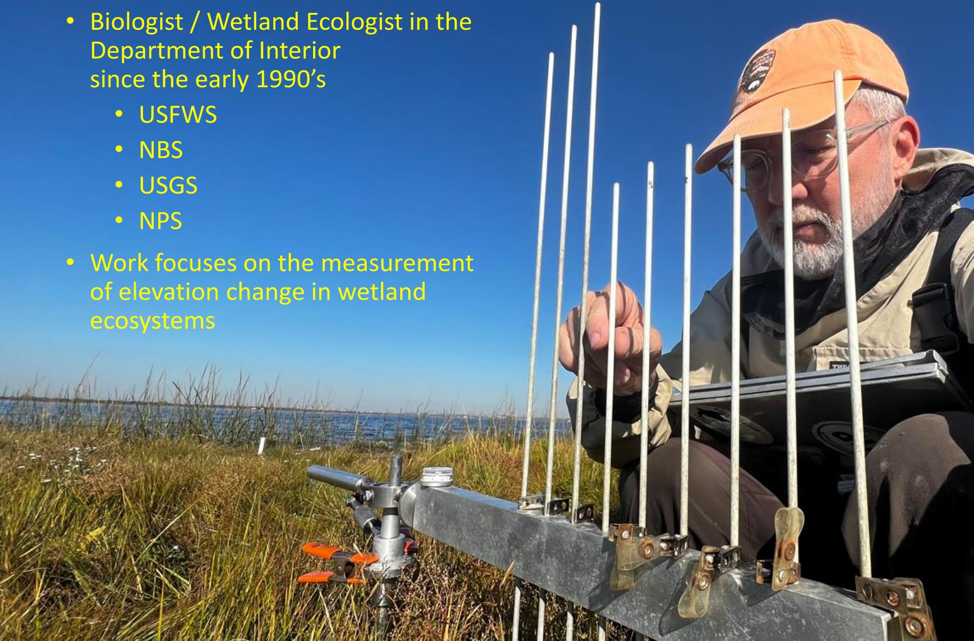
Wetlands grow vertically in response to sea level rise (SLR). The change is very small from year to year (mm) and a simple mechanical instrument, called the Surface Elevation Table (SET), was developed in early 1990's to monitor these small changes.
